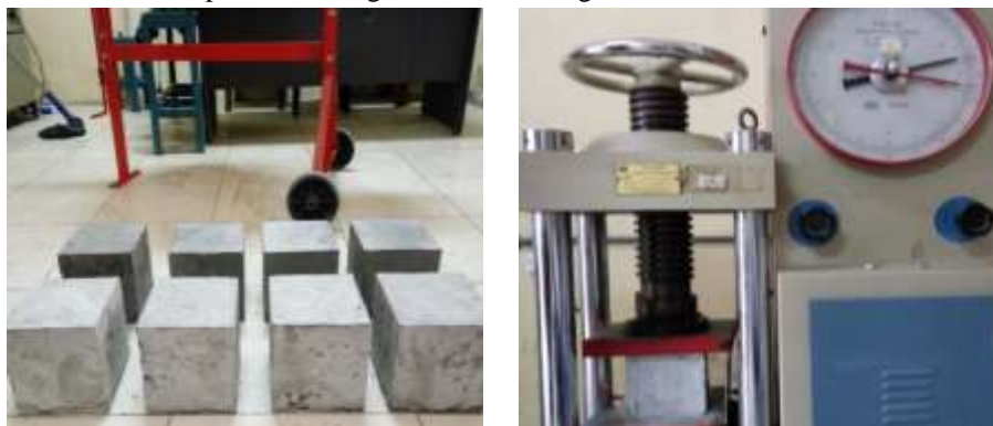
Figure 3. Testing conducted for the compressive strength
