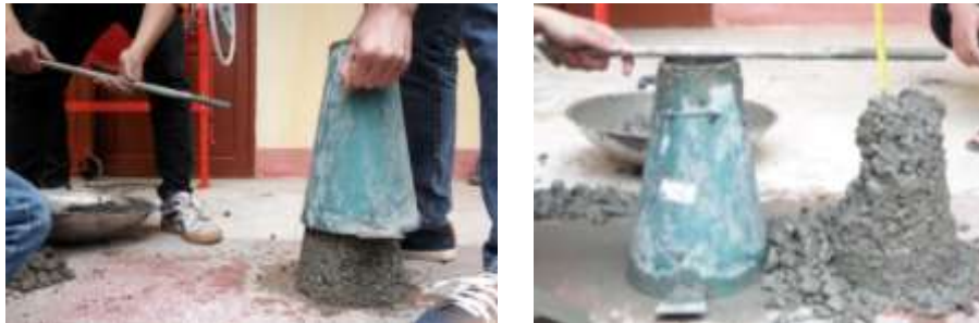
Figure 2: Slump test conducted for the study in this paper
